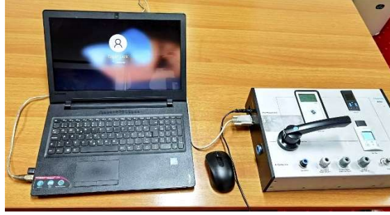
Figure 1: Connection of computer with Air Box measuring device
