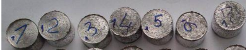
Figure 2. Compacted buttons made from metal powders.
