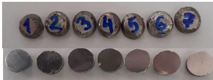
Figure 4. Mini-ingots casts and prepared for examination.
