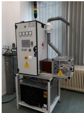
Figure 1. Melting equipment in inert atmosphere by levitation equipped with medium frequency converter.
