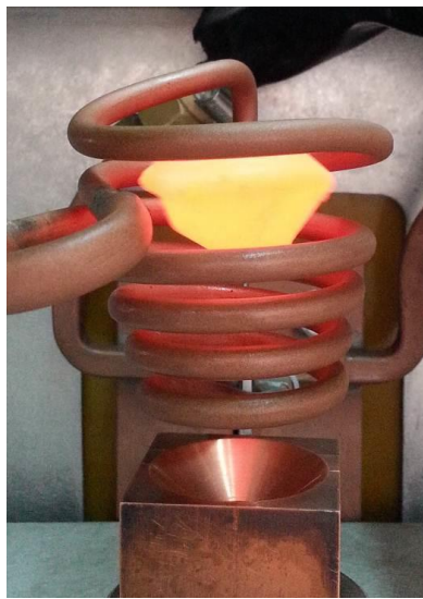
Figure 3. Image during the levitation melting process of the Mg-Zn-Y alloy button inside the inductor coil.
