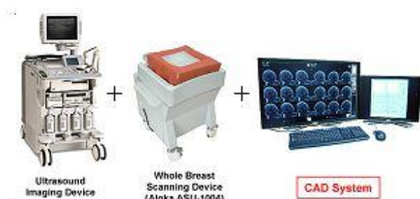
Figure 1. An overall system for breast cancer screening using ultrasound images. The system consists of an ultrasound imaging device and a whole-breast scanning device for whole breast volumetric data acquisition. A workstation is also included for the purpose of pre-processing and analysis of the images acquired by the scanning device from the patient and as a viewer for the visualization of the images along with the CAD results [28].
