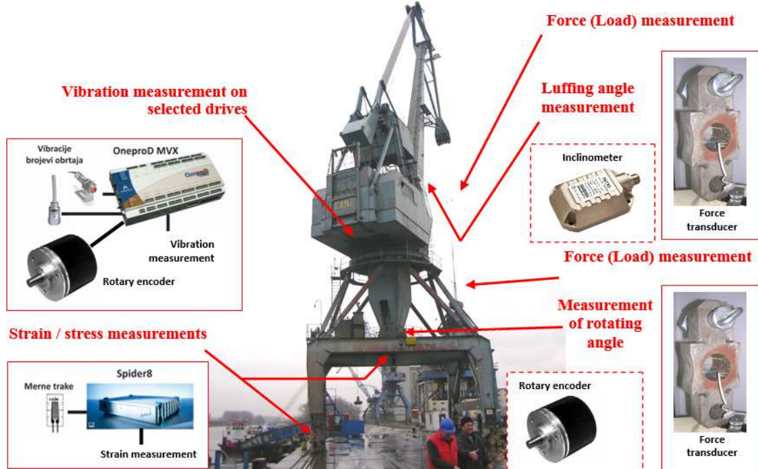
Figure 2. Measurement points at the crane
