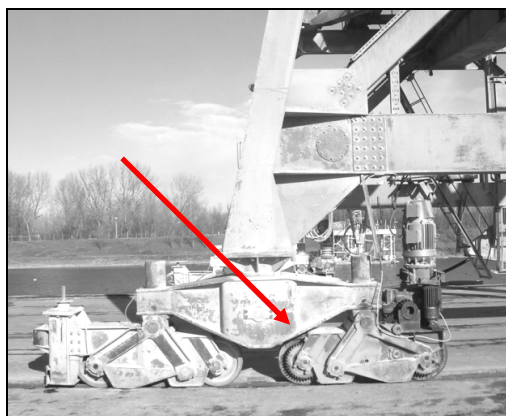
Figure 4. Recommended instrumentation (putting the measuring shaft instead of the rocker arm shaft with wheels)
