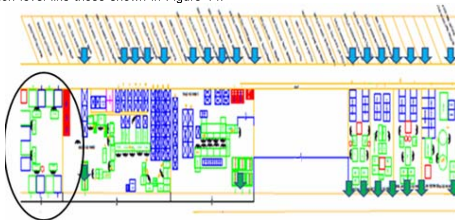
Figure 15. Input (blue arrows) and new output (green arrows) of the materials from the assembly lines
