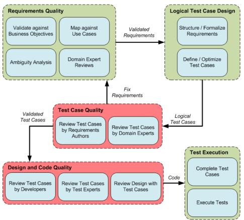
Figure 4. Requirements-based testing process flow
